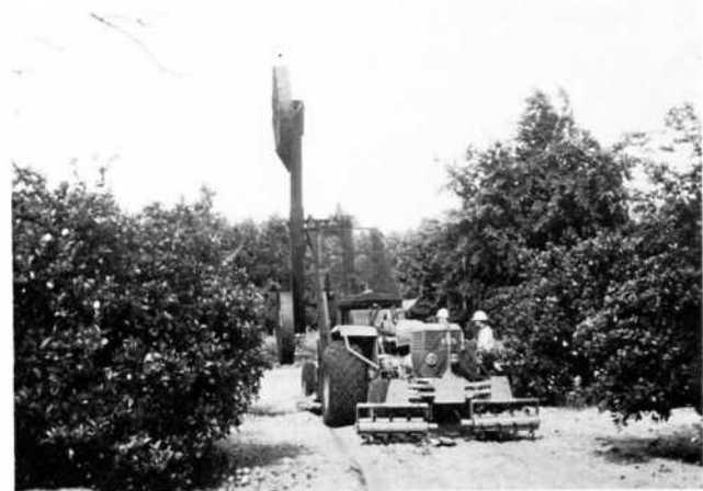
FIG. 2 Rotating boom air shaker using aircraft propellers to produce cyclic pulses of air on trees for fruit removal.
