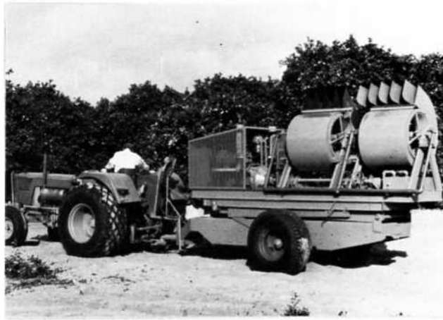
FIG. 1 Oscillating air shaker using two centrifugal fans to produce high velocity air streams for fruit removal. Vanes in air outlets direct the air streams to converge at 2.4 m.
