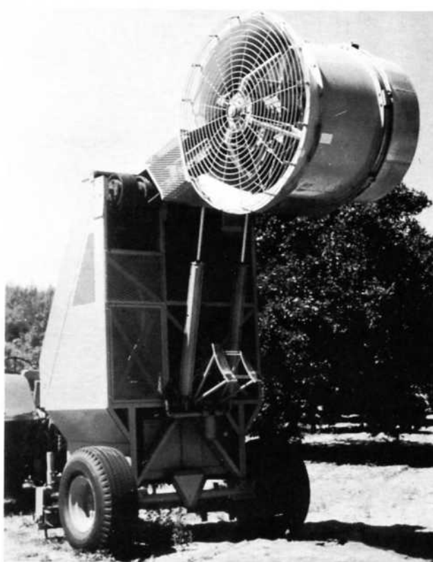
FIG. 5 Conical scan air shaker with fan in elevated position for reaching tops of tall trees. The shielded air inlet to fan is shown.
