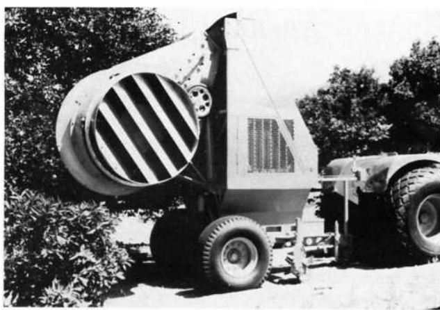
FIG. 4 Prototype air shaker using conical scan concept with fan at lowest position. The rotatable air director assembly with fixed vanes that direct the air is shown.
