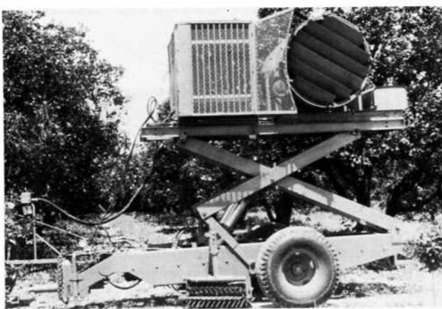
FIG. 3 Conical scan air shaker using a vane-axial fan and rotatable air director assembly to produce a cyclic pulse of high velocity air for fruit removal.
