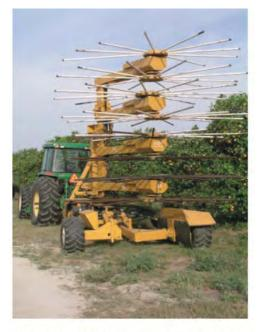
While the T-CS system does not harvest and catch Figure 8. Tractor-drawn canopy shaker. the fruit as efficiently as the CCSC system, it provides a more efficient alternative to hand harvesting in non-uniform groves. The Oxbo Corporation has been working to develop a "pick-up" machine to work in conjunction with a T-CS unit. As of the beginning of the 2008 harvest season, a commercial pick-up machine has not been perfected.
