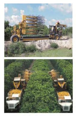
Figure 7. Continuous canopy shake-and-catch harvesting system side-view (top) and pair showing fruit conveyance and collection (bottom).
