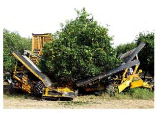
Figure 9. Trunk shake-and-catch harvesting system.
