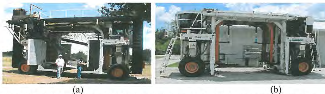
Fig. 5 a) The MaQtec harvester 2011 before modification. b) The MaQtec harvester converted into a mobile mechanical harvester test station.
