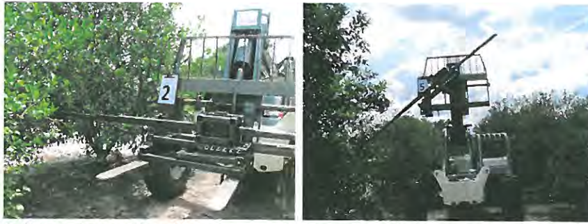
Fig. 8 a) Deflection and bending stress test rig mounted on the Terex telehandler with a perpendicular canopy placement. b) The test rig with at a 45-degree inclination angle.
