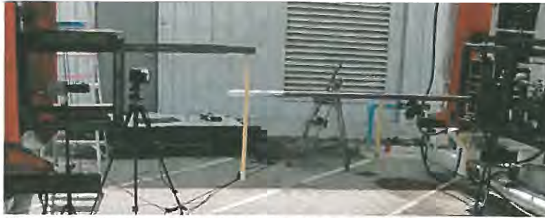
Fig. 6: The research-based mechanical harvester component and evaluation system with the present pivoting tine rig and a branch-bending stress and deflection evaluation system.
