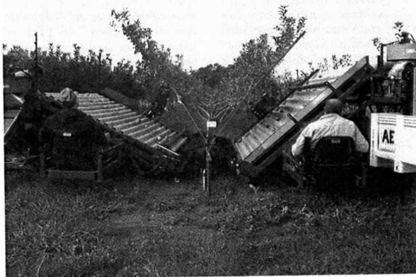
Fig. 2. Rear view of USDA-ARS experimental apple harvester in a “Y” trellised planting. Operators position rapid displacement actuators on scaffold to effect fruit removal. Apples are caught by “soft” moving conveyors and automatically placed in bins.
