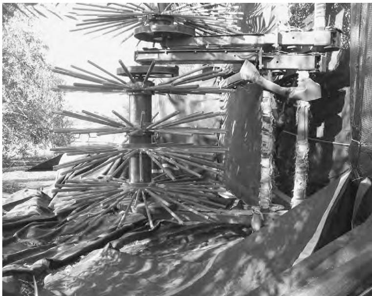
**Fig. 2. Vertical drum and horizontal rod radial distribution set-up for the lowest drum of the olive canopy shaker used during experimental tests on ‘Manzanillo’ table olives at the University of California Lindcove Experimental Station at Exeter in 2006. The harvester originated as an AgRight (Madera, CA)/Korvan (Lynden, WA)-engineered design prototype and has been modified by Dave Smith Engineering (DSE, Exeter, CA).**
