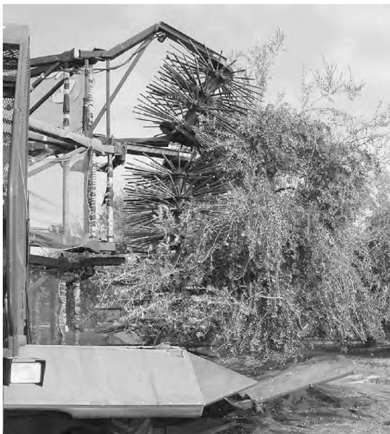
**Fig. 1.** Experimental olive canopy shaker used during tests on ‘Manzanillo’ table olives at the University of California Lindcove Experimental Station at Exeter in 2006. The harvester originated as an AgRight (Madera, CA)/Korvan (Lynden, WA)-engineered design prototype and has been modified by Dave Smith Engineering (DSE, Exeter, CA).
