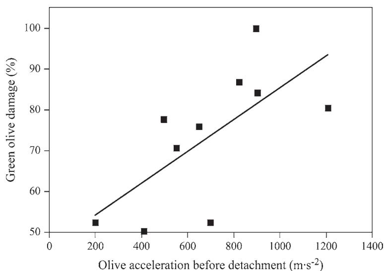
**Fig. 5. Measured acceleration of immature green ‘Manzanillo’ olive fruit before detachment from the canopy with stereo video cameras and computer software versus actual green olive damage induced by the experimental olive canopy shaker. The harvester originated as an AgRight (Madera, CA)/Korvan (Lynden, WA)-engineered design prototype and has been modified by Dave Smith Engineering (DSE, Exeter, CA); 1 m = 3.2808 ft.**
