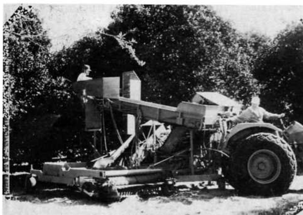
FIG. 4 Direct-loading, offset pickup machine in field operation.
