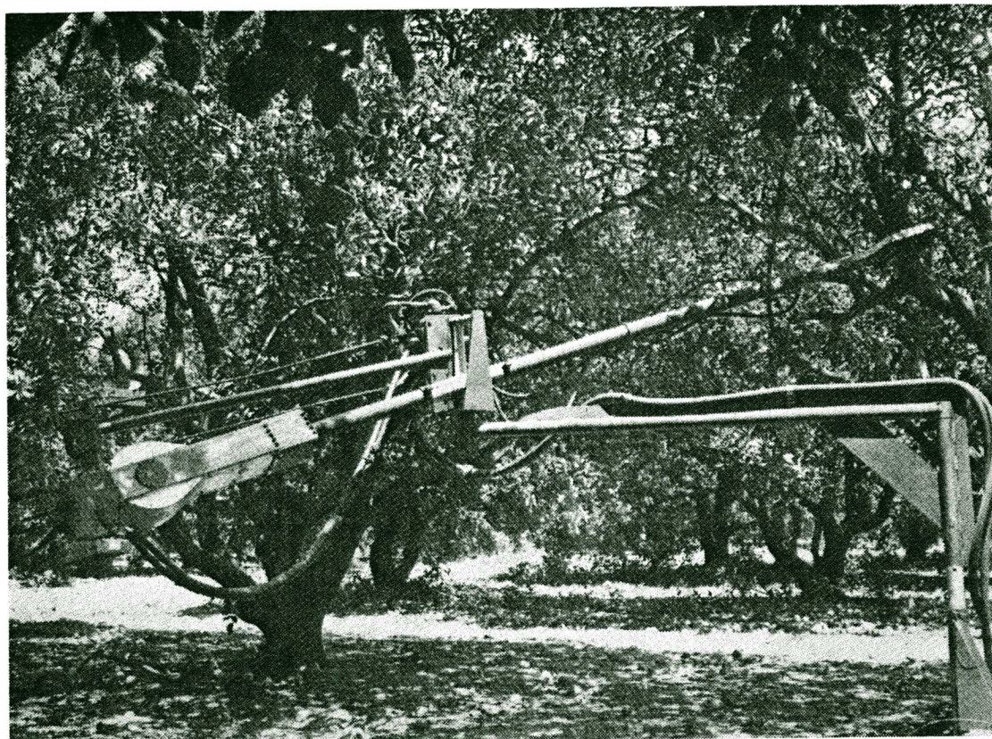
Figure 1.—Inertia tree shaker used to harvest citrus. A rotating eccentric weight of 85 pounds produces the shaking action.
