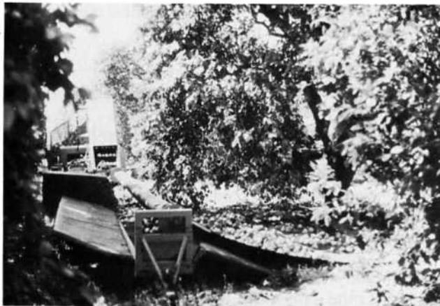
Fig. 2—Rollout fruit collector with canvas extended under the tree and loaded with oranges.
