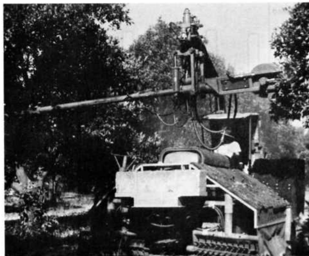
Fig. 1—Tractor-mounted sliding crank limb shaker used in length of stroke experiment.
