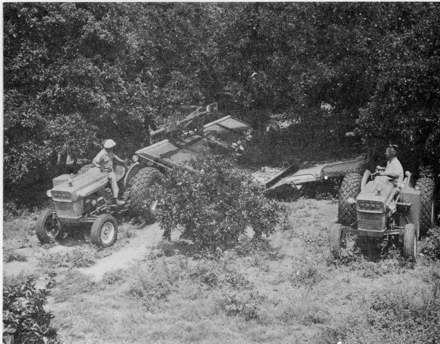
Fig. 1.--Catching frames being positioned around a tree in the tree shaker and catching frame harvest system.
