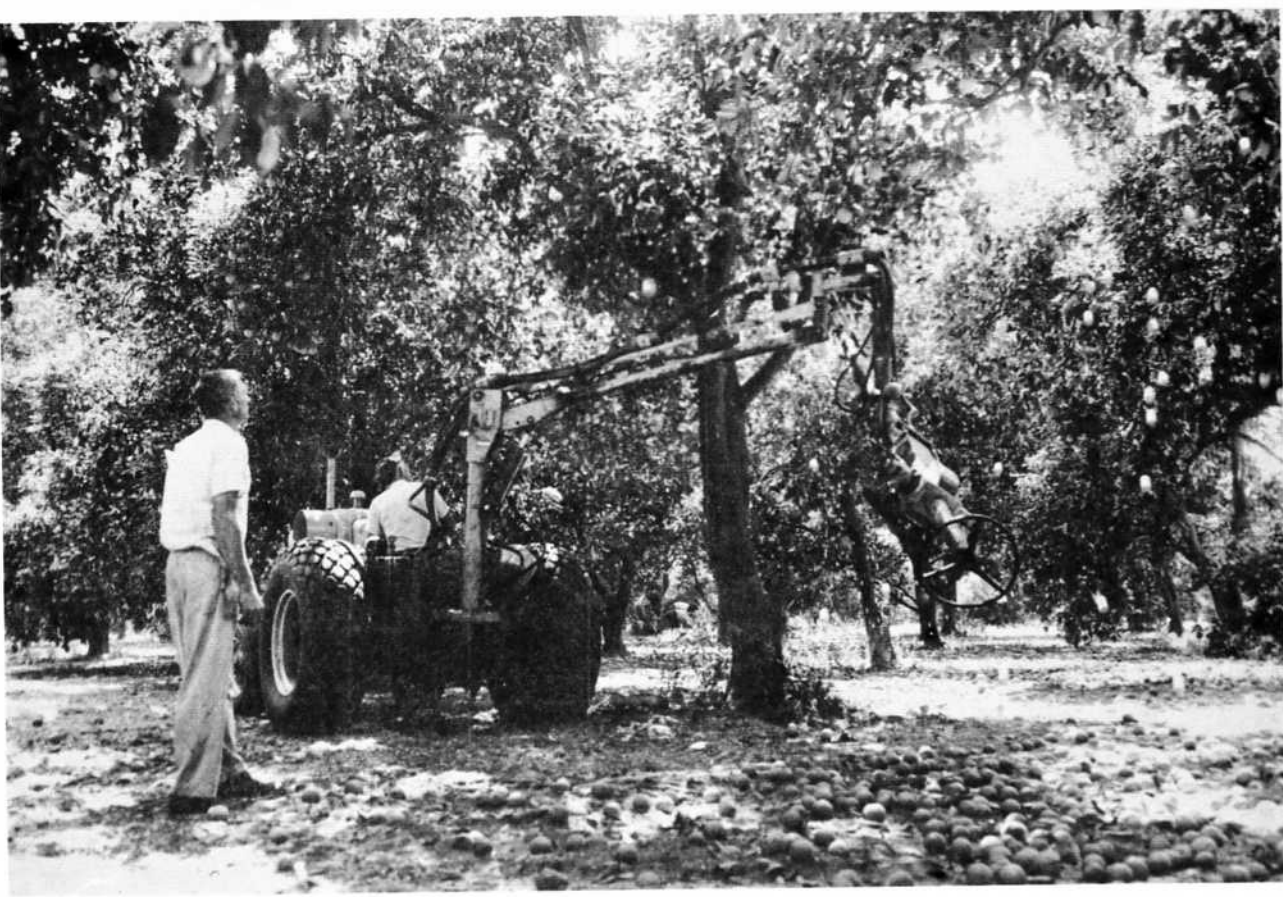
Fig. 3.--Tractor-mounted tree shaker being used to shake fruit onto the ground. This shaker is available commercially.
