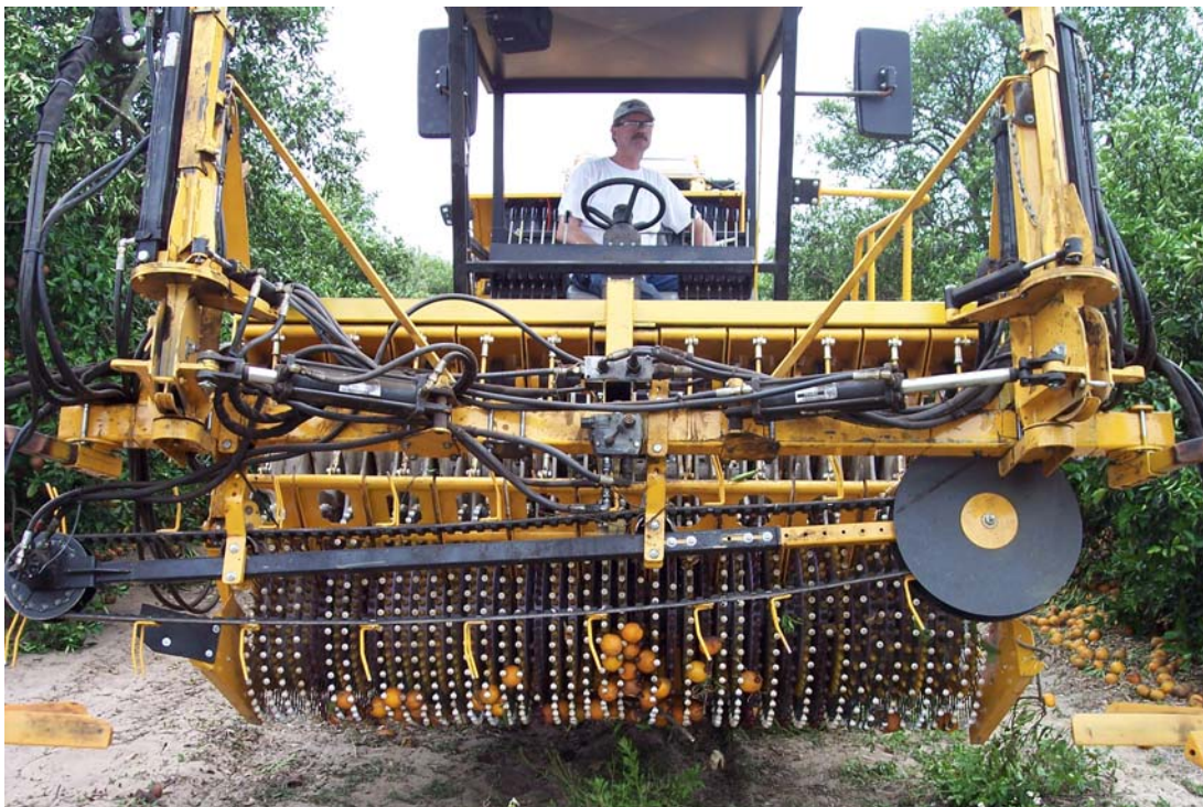
Figure 5: Closer view of the picking assembly and trash throwing belt
