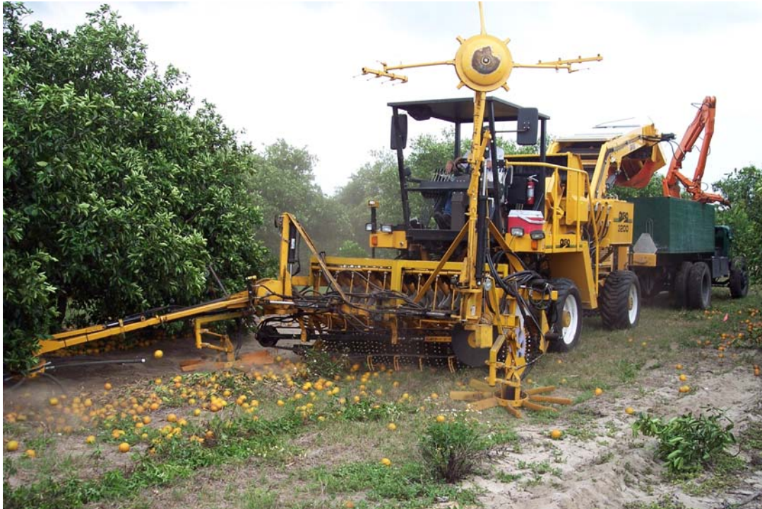
Figure 4: The modified OXBO pick-up machine
