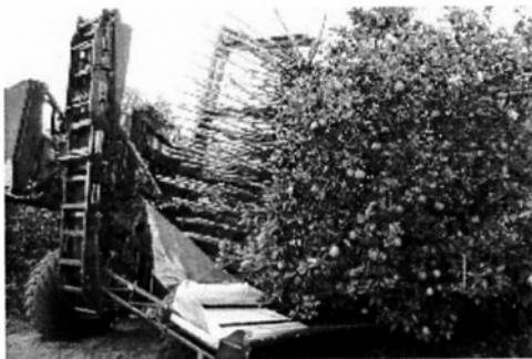
Figure 1. Canopy Shaker Design for Mechanical Citrus Harvester 1
