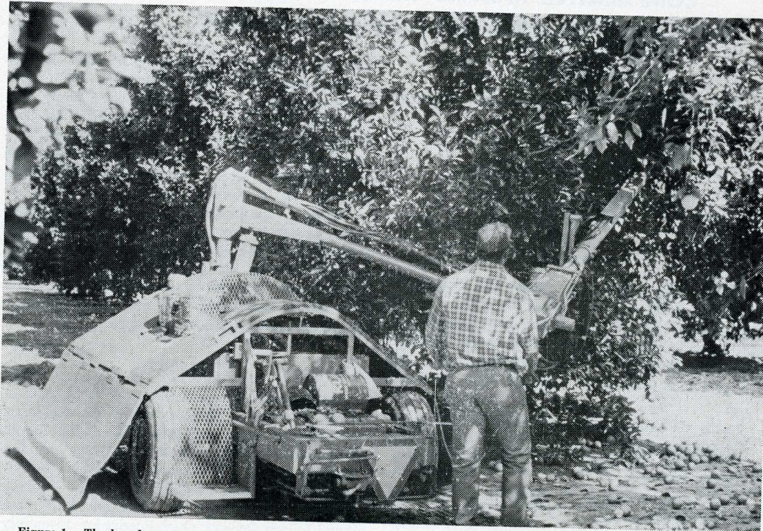
Figure 1.—The low frequency, large amplitude inertia type limb shaker used in these harvest tests.
