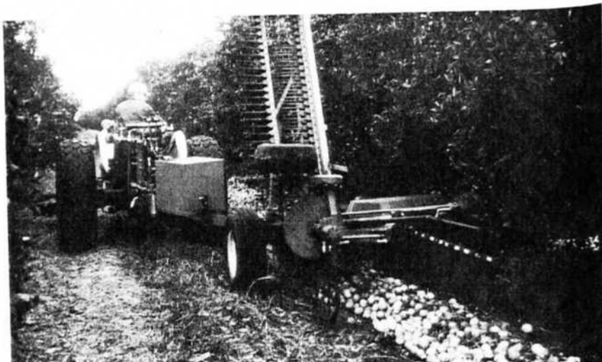
Fig. 1. Tractor-pulled windrow rake. This rake can be adjusted to form a center row or drip-line windrow of fruit.
