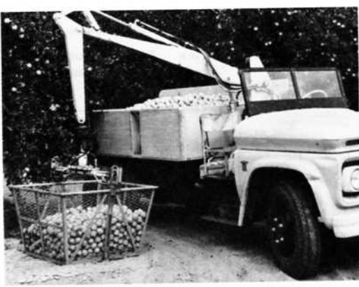
Fig. 3 Loader-Boom on High-Lift Truck Handling a Wire Basket
