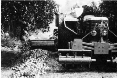
Fig. 6 Drip-line Pickup Machine
