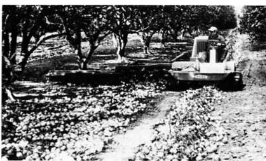
Fig. 5 Windrow Rake Forming Double Windrow for Center Drive Pick-up
