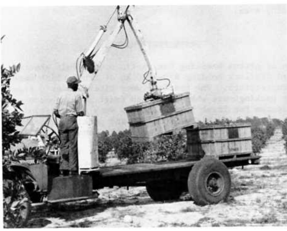
Fig. 2 Pallet Bin Handling With a Loader-Boom
