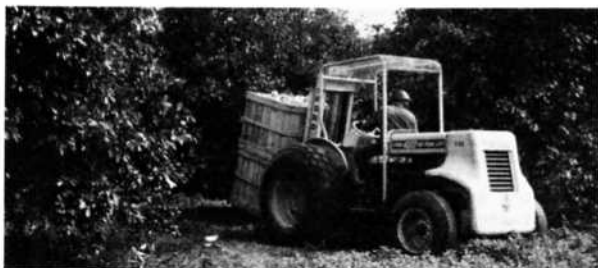
Fig. 1 Pallet Bin Handling With Tractor Fork-lift
