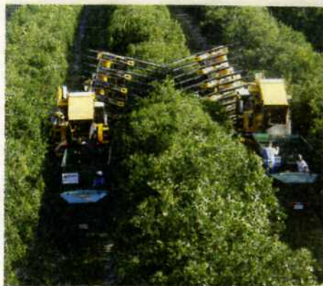
The trunk shake and catch (top) and the continuous canopy shake and catch harvesters were developed by the Florida Department of Citrus and brought into commercial use in the 1990s.
