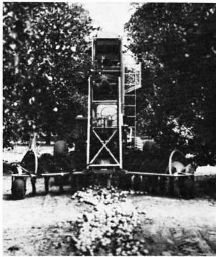
FIG. 1 Front view of USDA experimental citrus pick-up machine.
