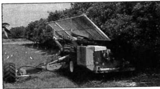
The Coe-Collier machine demonstrates the Trunk Shake and Catch system (TSC).
