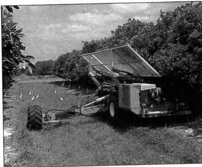
◀ The trunk-shake-catch, demonstrated by the Coe-Collier machine.
