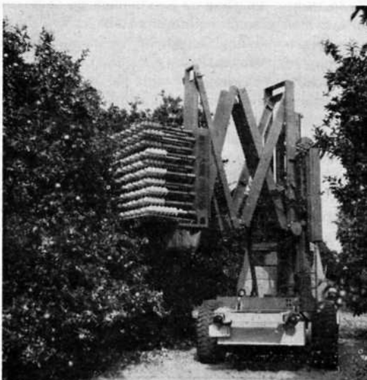
Figure 1.—Positioner lowered and ready for entry into tree.
