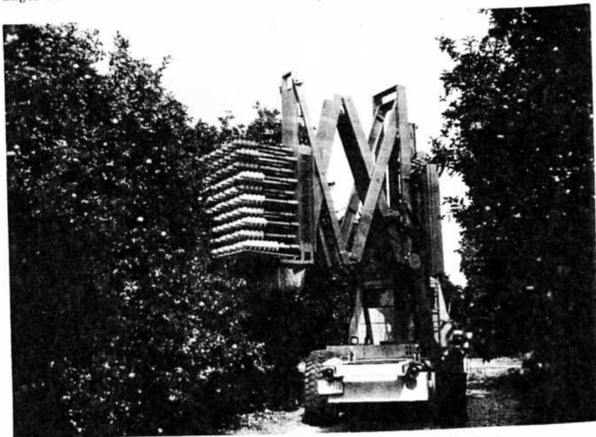
Figure 1. Positioner lowered and ready for entry into tree.
