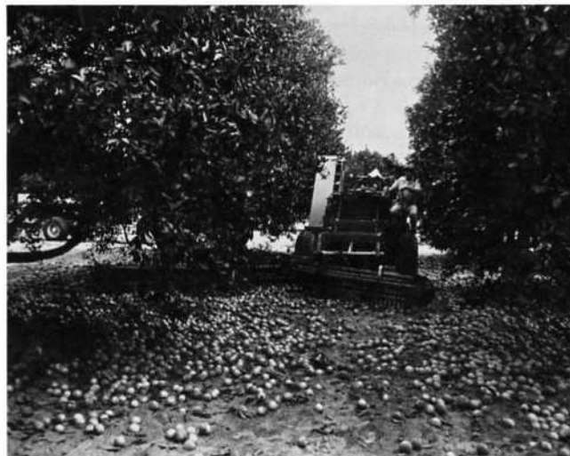
FIG. 1 The rake-pickup machine operating in the semicommercial harvest system.
