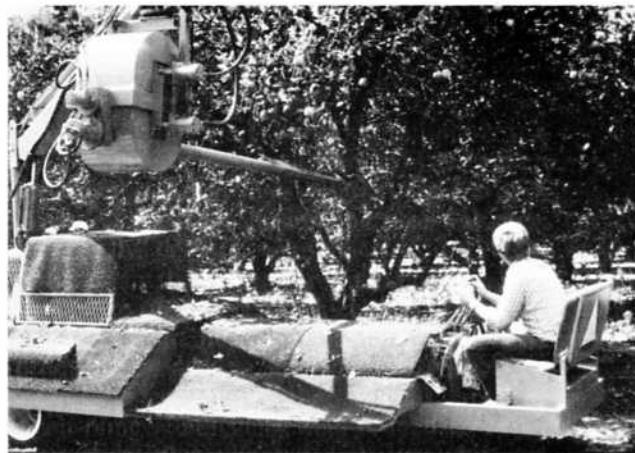
FIG. 1 Limb-shaker unit with full-powered positioning mechanism.
