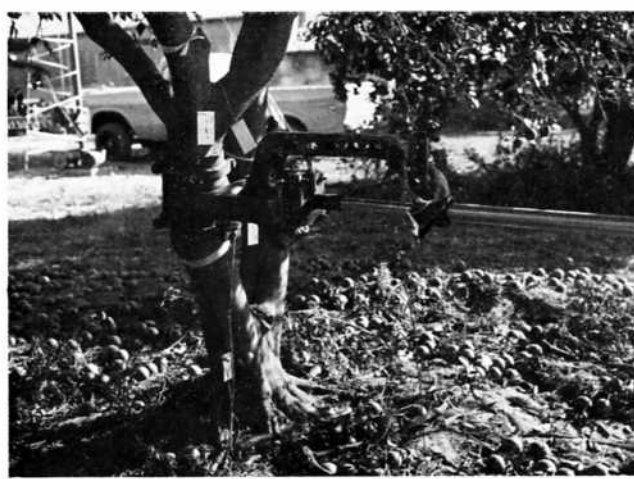
FIG. 2 Force transducer and accelerometer attached to the limb and shaker.
