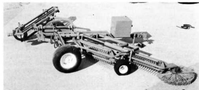
FIG. 4 Tractor-drawn rake in final stages of construction.
