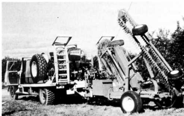
FIG. 6 Transport system for tractor-drawn windrow rake (dripline arrangement).
