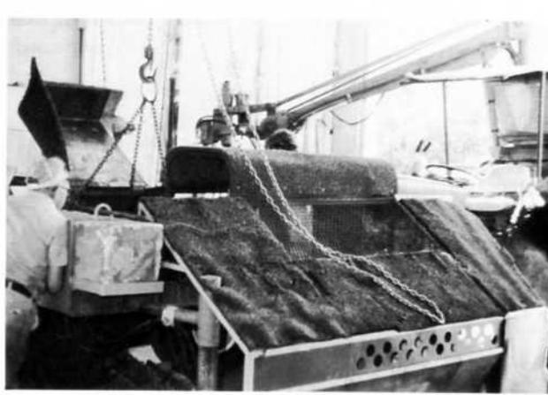
FIG. 6 Overhead hoist attached to the front counterweight assembly for attachment to the tractor.
