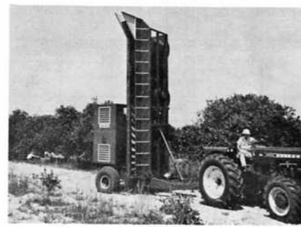
FIG. 11 FMC-2 showing "wobble plates" in air outlet.
