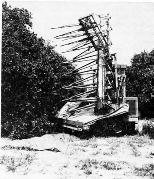
Fig. 1. Vertical foliage shaker used in 'Valencia' harvest experiment.
