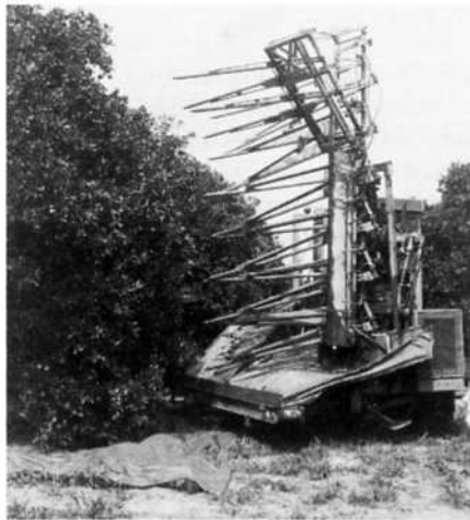
FIG. 1 Vertical foliage shaker used in Hamlin- and Valencia-orange harvesting experiments.
