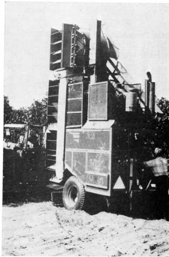
Fig. 1. AREC air shaker with 3 vane-axial fans (48 in.) and 2 engines.
