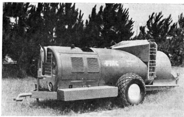
Fig. 1. FMC Model 757 CP sprayer with double oscillating citrus volute and powered by auxiliary engine.
