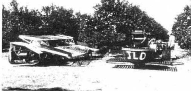
Figure 3—Rear view of Compton shake-catch harvester. Shake/deflector unit is at left of tree row and receiver unit is at right of tree row.
