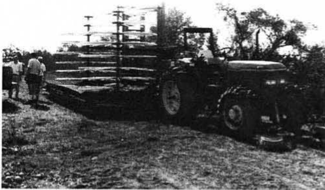
Figure 2—Front view of USDA canopy shaker with catchframe as operated in tests 5 and 6.
