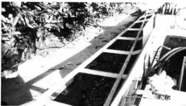
Figure 4—Rear view of Compton receiver unit. Dump pan is at left and longitudinal conveyor is at center.
