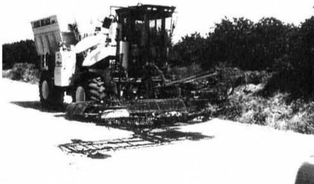
Figure 6—Front view of Agricultural Machines pickup machine as mounted on the Pixall Big Jack®.
