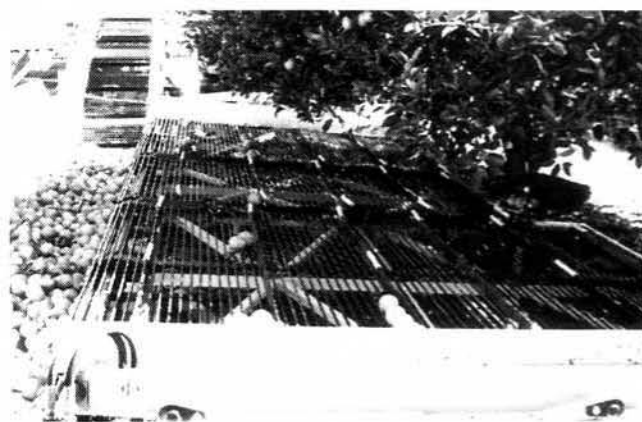
Figure 7—Front view of Compton rebuilt receiver unit showing cross conveyors at right which moved fruit to the longitudinal conveyor at left.
