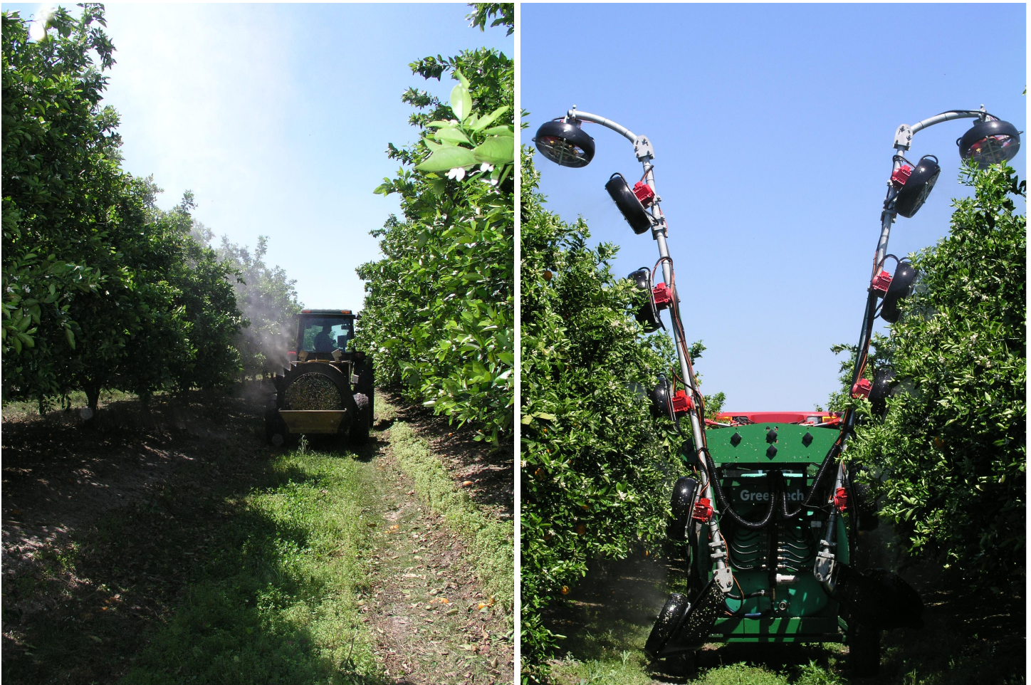
Fig. 1. The air-blast (left panel) and 'GreenTech' (right panel) sprayers used in these studies.
