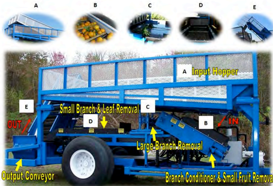
Fig. 14. Different components of trash removal system
