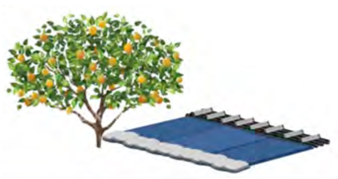
Fig. 9. Catch plates contour to the trees. The fruit is conveyed to the pinch-rollers, and then conveyed into the elevator positioned on the goat truck by smaller width conveyors.
