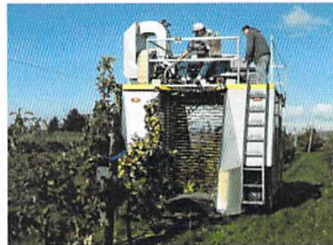
An over-the-row small fruit harvester passes over cider apple trees at WSU Mount Vernon. (Photos by Carol Miles, WSU)
