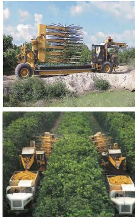
Figure 7. Continuous canopy shake-and-catch harvesting system side-view (top) and pair showing fruit conveyance and collection (bottom).
