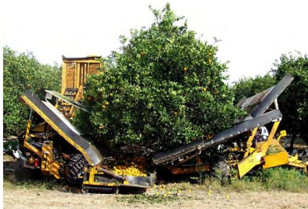
Figure 9. Trunk shake-and-catch harvesting system.
