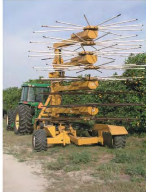
While the T-CS system does not harvest and catch the fruit as efficiently as the CCSC system, it provides a more efficient alternative to hand harvesting in non-uniform groves. The Oxbo Corporation has been working to develop a “pick-up” machine to work in conjunction with a T-CS unit. As of the beginning of the 2008 harvest season, a commercial pick-up machine has not been perfected.
